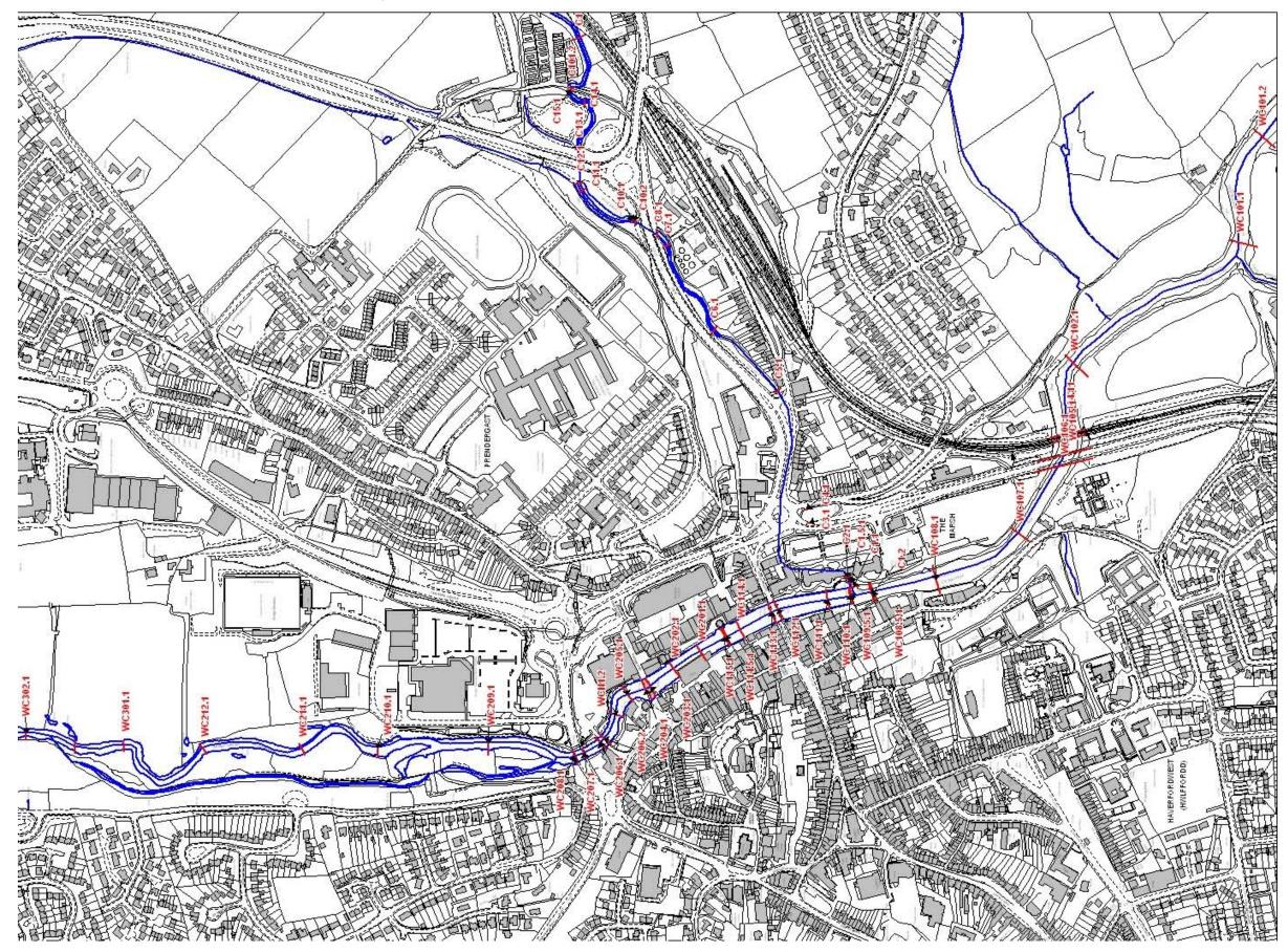
Figure 6.1 Cross Section locations in 1D model of Western Cleddau & Cartlett Brook, Haverfordwest
